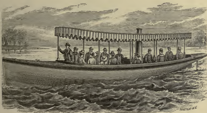
FIG. 96.—30 FT. LAUNCH, WITH FOUR HORSE POWER ENGINE.
